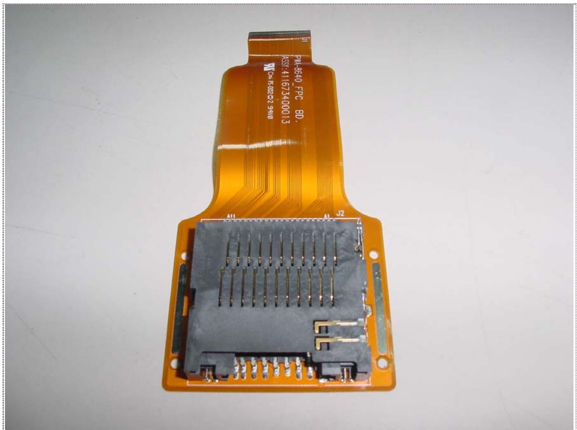
Component Side View of Memory
